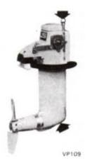
Remove the oil dipstick. Remove the plug underneath the propeller gear housing and let the oil drain off. Install the plug with its O-ring. Fill oil through the dipstick hole. The oil level shall be within the dipstick marks. NOTE! Do not fill oil above the upper oil dipstick mark. Concerning the choice of oil, see "Technical Data", Page 30.
