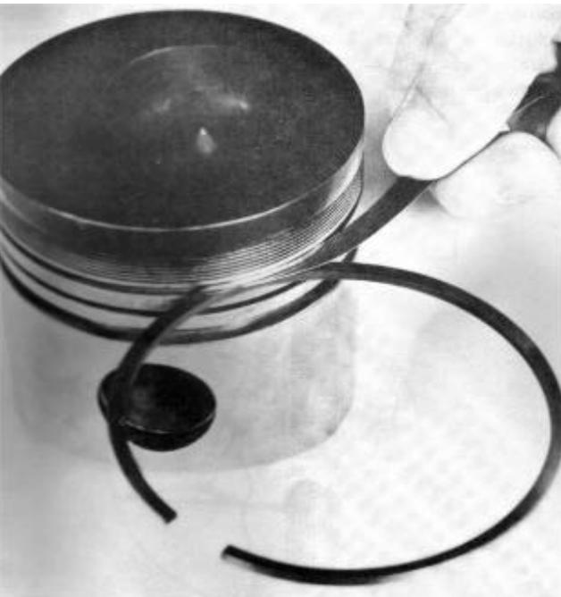
**43.** Fit the piston rings with the help of piston ring pliers. Start with the oil scraper ring in the lowest groove. The oil scraper ring can be fitted either way. Continue with the compression ring which is marked "TOP" on one side. This marking shall face upwards when fitted. The piston ring with the chromium insert is fitted last and can be fitted either way.
