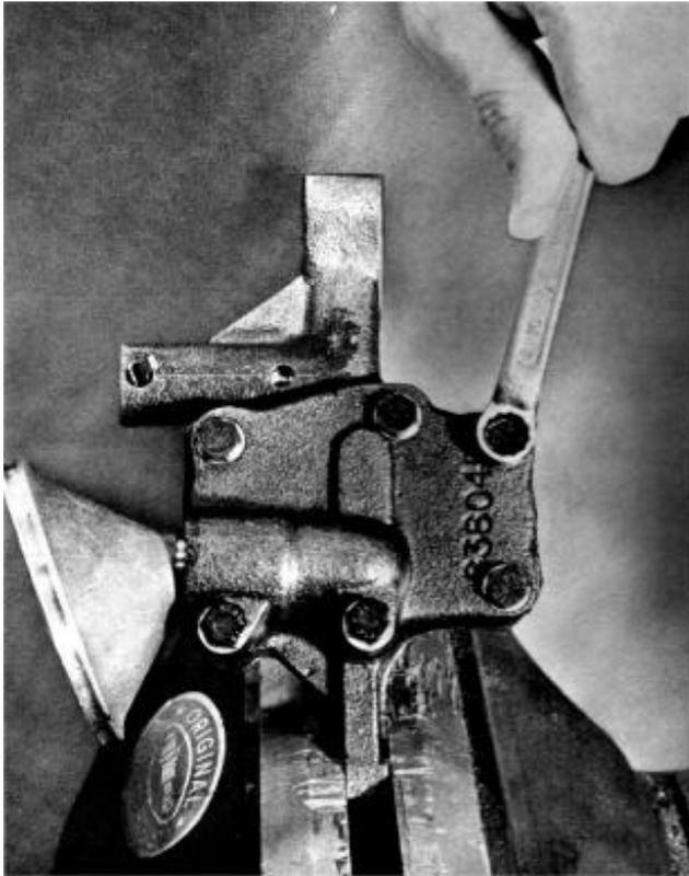
22. Remove the gearwheel from the housing. Remove the split pin for the reduction valve. Remove washer 1, spring 2 and piston 3. Clean and replace damaged parts. Assemble the lubricating oil pump in the reverse order. Note! Fit a new gasket 4 between the housing and the cover. Fix the wire mesh 5 in position with the steel wire 6 and finally lay the key 7 in position and tighten the gearwheel 8.
